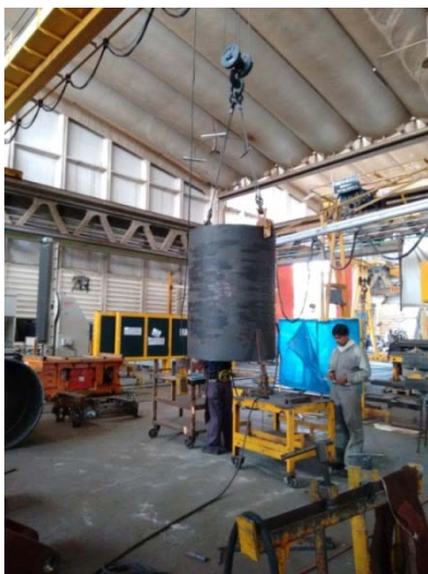
Fig. 3: Current method of full welding process
