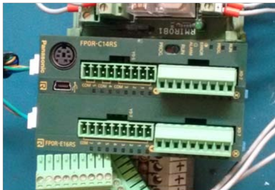
Fig. 14: A PLC unit used in the welding automation
