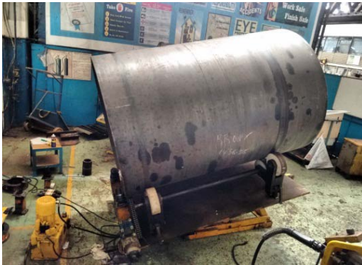
Fig. 13: Component placed on the tilted fixture
