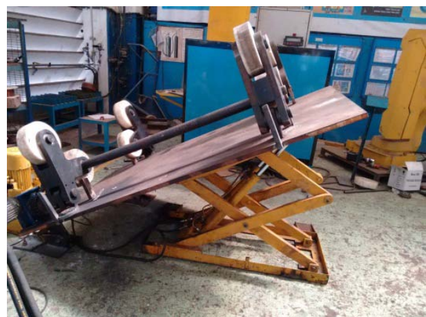
Fig. 12: Hydraulic cross-lift tilting the fixture at 30
